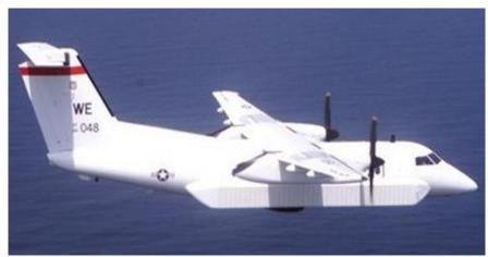
The E-9 twin turbo prop aircraft is used as a surveillance platform. Ensuring the Gulf Coast waters are clear of boaters and aircraft during live missile test. The E-9 aircraft will be seen daily in the Tyndall terminal area and special use airspace.
