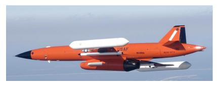
Tyndall utilizes a ground launched, land and water recoverable subscale aerial target for live missile training. It is 20 feet in length and has a wingspan of 12 feet. It travels at speeds from 250 knots up to .95 mach and operates at altitudes from 50 to 50,000 feet. But can normally be found between 15,000 and 25,000 at around 300 knots. These drones deploy frequently within restricted area 2905A.
