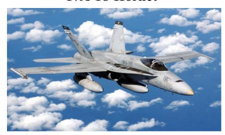
The McDonnell Douglas F/A-18 Hornet is a twin-engine supersonic, all-weather carrier-capable multirole combat jet, designed to dogfight and attack ground targets.
