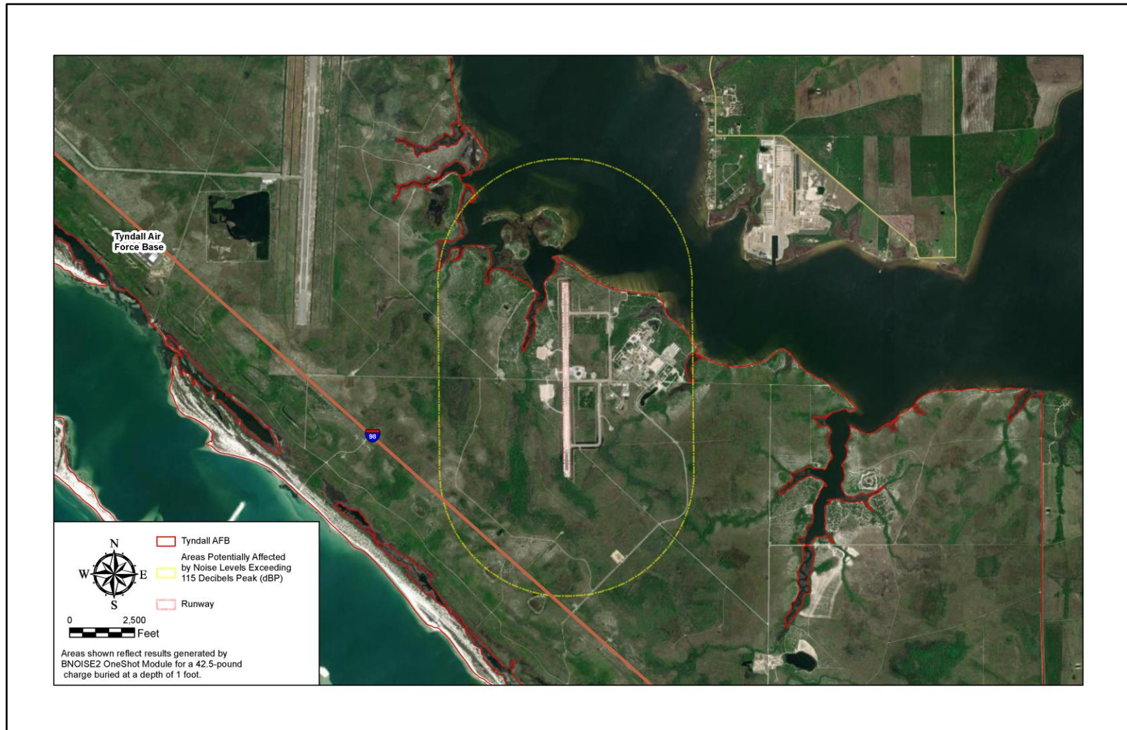
Figure 3-5. Areas Potentially Affected by Noise Levels Exceeding 115 dBp Generated by Explosive Charge Detonations During Proposed CSTR Training
